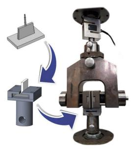
Figure 3. The special grip for the rib pull-off tests.
