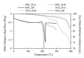
**Figure 8.** Differential scanning calorimetry (DSC) and thermogravimetric analysis (TGA) curves for the three different plates.
