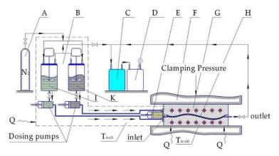
**Figure 1.** Scheme of the T-RTM process (A—nitrogen source; B—dosing unit; C—cold trap; D—vacuum pump; E—dynamic mixing head; F—mold carrier; G—metal mold; H—textile preform; I—tank with  $\varepsilon$ -caprolactam + initiator; K—tank with  $\varepsilon$ -caprolactam + activator [8].
