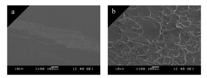
Figure 6. Scanning electron microscopy tests (100 × magnification): (a) non-welded; (b) welded areas.
