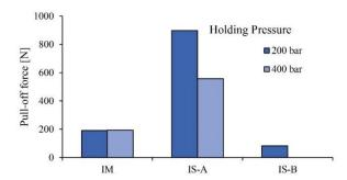
**Figure 7.** The pull-off force for the three different plates (IM—injection-molded plates; IS-A—magnesium catalyst-based in situ polymerization plates; IS-B—Brüggemann AP-NYLON-based in situ polymerization plates).
