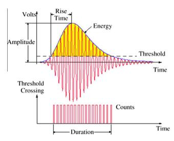
**Fig. 5.** The definitions for acoustic-emission parameters [37]. (For interpretation of the references to colour in this figure legend, the reader is referred to the web version of this article.)
