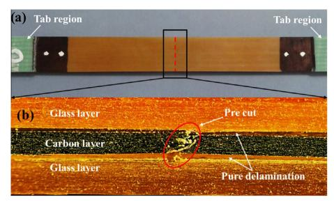
**Fig. 8.** (a) Top and (b) side view of a typical delaminated  $[G_4/C_8/G_4]$  type specimen with TR30 carbon. (For interpretation of the references to colour in this figure legend, the reader is referred to the web version of this article.)
