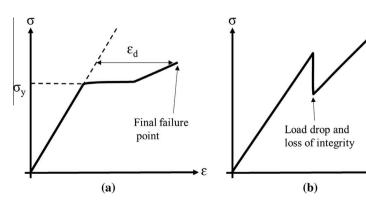
Fig. 1. Schematic of the typical stress-strain graph of (a) a thin-ply hybrid with pseudo-ductility and (b) a conventional hybrid with catastrophic delamination.
