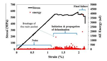
**Fig. 9.** Stress–strain and AE event energy for pure delamination in a typical  $[G_4/C_8/G_4]$  with a pre-cut in the TR30 carbon layer. (For interpretation of the references to colour in this figure legend, the reader is referred to the web version of this article.)
