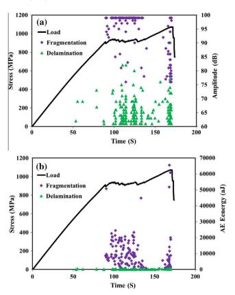
**Fig. 12.** Distribution of (a) amplitude and (b) energy of the AE events for a typical MR40/S-glass specimen. (For interpretation of the references to colour in this figure legend, the reader is referred to the web version of this article.)
