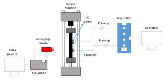
Fig. 4. Schematic of the experimental setup. (For interpretation of the references to colour in this figure legend, the reader is referred to the web version of this article.)
