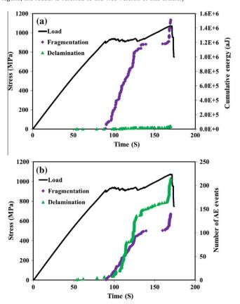
**Fig. 13.** The cumulative of (a) AE energy and (b) number of the AE events in each class of the AE signals in a typical MR40/S-glass specimen. (For interpretation of the references to colour in this figure legend, the reader is referred to the web version of this article.)
