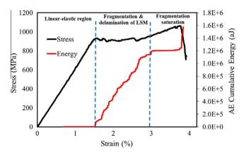
**Fig. 7.** Stress–strain and cumulative AE energy distribution for a typical MR40/S-glass hybrid specimen. (For interpretation of the references to colour in this figure legend, the reader is referred to the web version of this article.)
