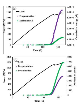
**Fig. 15.** The cumulative of (a) AE energy and (b) number of the AE events in each class of the AE signals for a typical 1TR30/S-glass specimen with one carbon ply. (For interpretation of the references to colour in this figure legend, the reader is referred to the web version of this article.)
