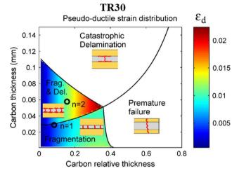
**Fig. 2.** Distribution of pseudo-ductile strain for  $[G_1/C_n/G_1]$  laminates made with MR40 and TR30 carbon, where (n = 1-3). (For interpretation of the references to colour in this figure legend, the reader is referred to the web version of this article.)
