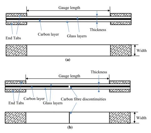
**Fig. 3.** Schematics of thin ply hybrid composite specimen types for tensile testing with (a) continuous and (b) pre-cut carbon layers. (For interpretation of the references to colour in this figure legend, the reader is referred to the web version of this article.)
