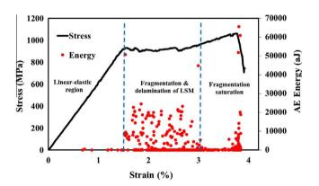
**Fig. 6.** Stress–strain and AE event energy distribution for a typical MR40/S-glass type specimen. (For interpretation of the references to colour in this figure legend, the reader is referred to the web version of this article.)
