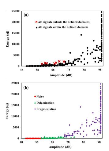
**Fig. 11.** Plots of amplitude and energy of the AE events for a typical MR40/S-glass specimen. (a) Before applying the defined boundaries in Fig. 10a. (b) After applying the defined boundaries. (For interpretation of the references to colour in this figure legend, the reader is referred to the web version of this article.)
