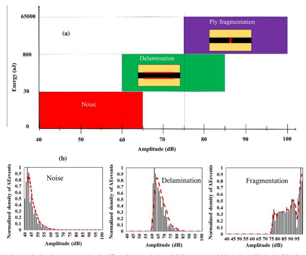
**Fig. 10.** (a) Event amplitude and energy ranges assigned to different damage mechanisms of ply fragmentation and delamination and (b) density of the AE events in the amplitude domain for a typical MR40 hybrid specimen (the red dash lines are moving average trend lines). (For interpretation of the references to colour in this figure legend, the reader is referred to the web version of this article.)
