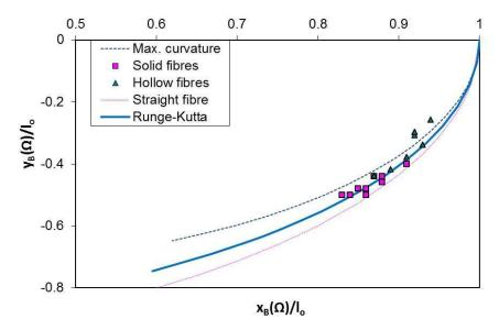
Figure 4 Measured coordinates of fibre end-points, boundary curves, and the fibre-end curve determined with the Runge-Kutta method
