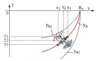
Figure 6 Three possible positions of the measured end-point sets (x, \*, o) and their average points (red, cyan, and blue  $\mathbf{O}$ ) and intersection points (black  $\mathbf{O}$ ) of the theoretical end-point curve and the coordinate lines of average points red and blue
