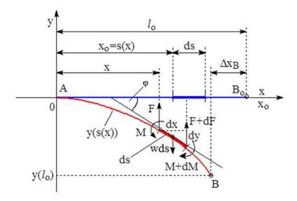
Figure 2 Schematic of the forces acting on an arc element of the deflected fibre  $(y_B=y(l_o))$
