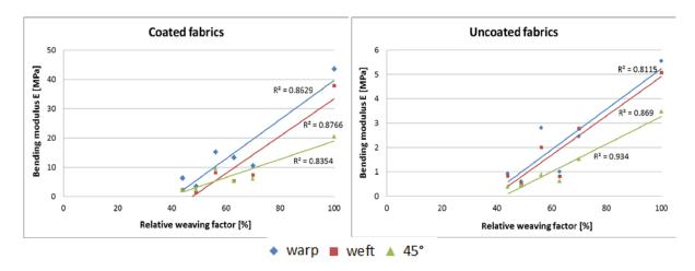
Figure 6: Bending modulus of the coated and uncoated fabrics in different directions depending on relative weaving factor measured by Flexometer
