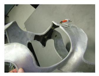
Figure 14. The composite corsette with the connector and built sensors
