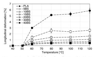
Figure 15. Longitudinal deformation of PLA and 5–10–15– 20–30–40 wt% basalt fibre reinforced composites with silane treatment
