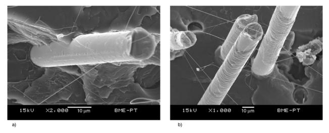
Figure 8. Cross-section of untreated (a) and treated (b), 15 wt% basalt fibre reinforced PLA composite
