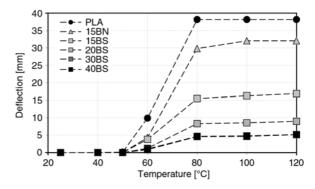
Figure 16. The deflection of the basalt fibre reinforced PLA composites
