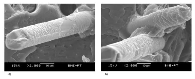
Figure 9. Cross-section of 20 wt% (a) and 40 wt% (b) silane treated basalt fibre reinforced PLA composite
