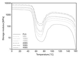
**Figure 12.** Storage modulus of amorphous PLA (PLA) and 5–10–15–20–30–40 wt% basalt fibre reinforced composites with silane treatment
