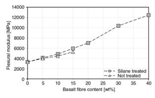
Figure 5. Flexural modulus of the basalt fibre reinforced PLA composites
