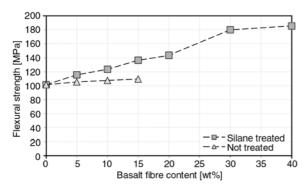
Figure 4. Flexural strength of the basalt fibre reinforced PLA compositesb
