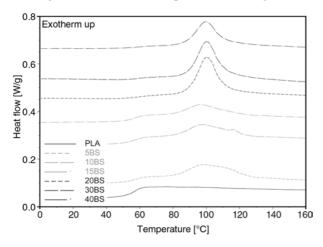
Figure 10. Cooling scan of 5–10–15–20–30–40 wt% basalt fibre reinforced composites
