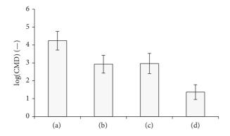
FIGURE 3: The homogeneity differences between injection molded test specimens: (a) original masterbatch, (b) modified masterbatch produced on a special extruder, (c) modified masterbatch produced on the LabTech corotating twin-screw extruder, and (d) compounded material.
