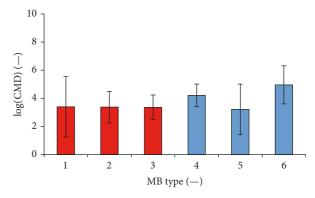
FIGURE 4: Inhomogeneity scores of the tested masterbatches in the first test series (1: Red Dye; 2: Red Organic; 3: Red Inorganic; 4: Blue Dye; 5: Blue Organic; 6: Blue Inorganic).
