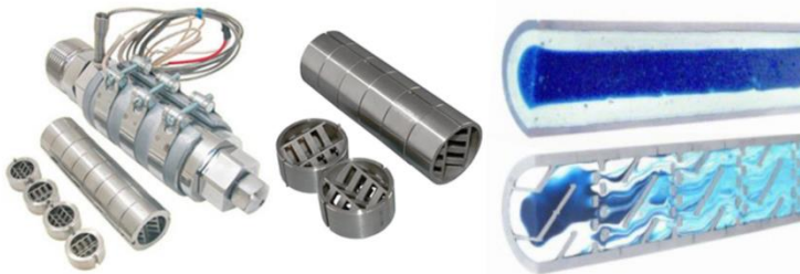
Figure 1. Stamixco injection molding static mixing nozzle with the elements (left); Empty nozzle provides no mixing (right top) and eight SMN mixing elements create homogeneous mixing in a short length (right bottom) [22].
