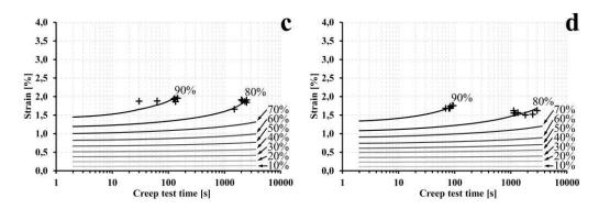
Fig. 6. Creep strain of 5wt% (a), 10wt% (b), 20wt% (c) and 30wt% (d) basalt fibre reinforced PLA at various static loading levels. The curves are averaged creep curves, while the cross means the breakage of the single specimens
