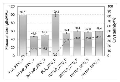
Fig. 10. Flexural strength of PLA and PLA based compounds injection molded into steel and PolyJet molds
