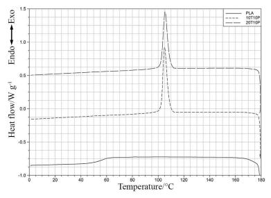
Fig. 3. DSC cooling scan of PLA and PLA based nucleated compounds registered at 5°C min<sup>-1</sup>
