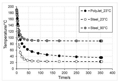
Fig. 2. The temperature of the molded part as a function of cooling time for the three different mold materials
