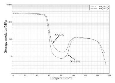
Fig. 5. Storage modulus of pure PLA injection molded into 23°C steel and PolyJet mold
