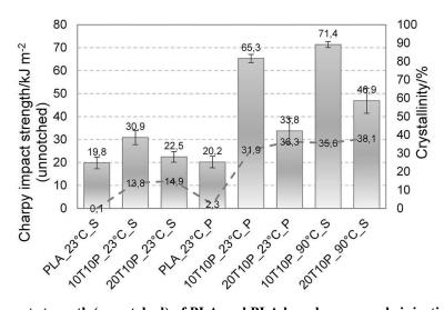
Fig. 14. Charpy impact strength (unnotched) of PLA and PLA based compounds injection molded into steel and PolyJet molds
