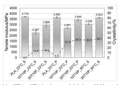
Fig. 11. Tensile modulus of PLA and PLA based compounds injection molded into steel and PolyJet molds
