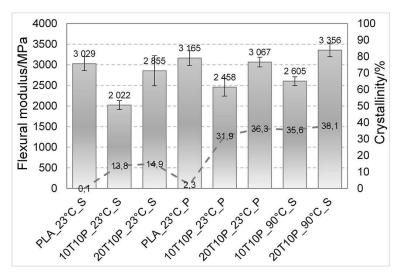
Fig. 12. Flexural modulus of PLA and PLA based compounds injection molded into steel and PolyJet molds
