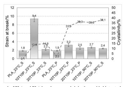
Fig. 13. Strain at break of PLA and PLA based compounds injection molded into steel and PolyJet molds
