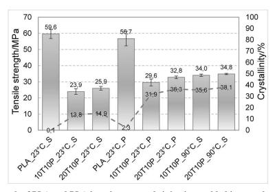
Fig. 9. Tensile strength of PLA and PLA based compounds injection molded into steel and PolyJet molds
