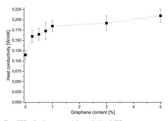
Figure 7 Effect of graphene content on the heat conductivity of pCBT
