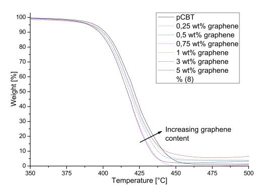
Figure 5 Thermogravimetrcical curves of graphene-modified pCBT samples
