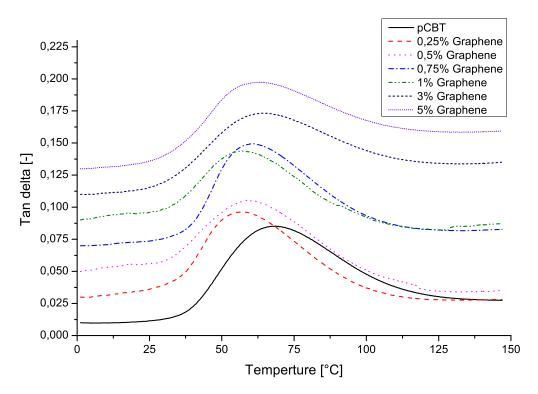
**Figure 3** Tangent delta vs. temperature curves of pCBT samples containing different graphene amount (curves shifted along the y axis for better visibility
