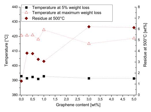
Figure 6 Thermal decomposing properties of graphene-modified pCBT samples
