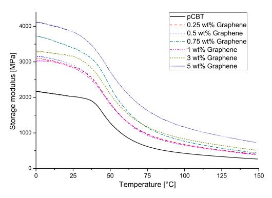
**Figure 4** Storage modulus vs. temperature curves of pCBT and pCBT nanocomposites containing different amounts of graphene
