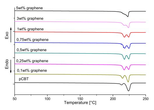
Figure 1 Melting DSC scans of graphene containing pCBT samples
