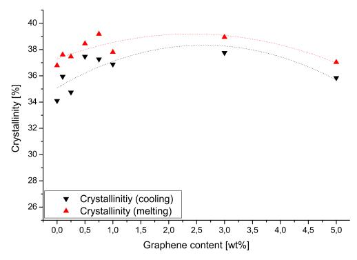
Figure 2 Crystallinity in function of graphene content
