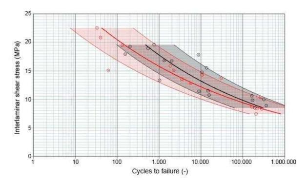
**Fig. 8.** S-N curves of the DNS fatigue tests (CF/EP – red, CF/MWCNT/EP – black)
