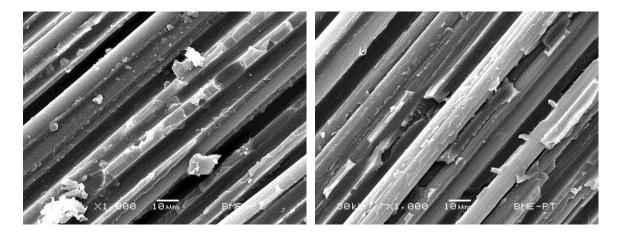
**Fig. 3.** SEM micrographs of the fracture surfaces of the static DNS specimens (CF/EP – left, CF/MWCNT/EP – right)
