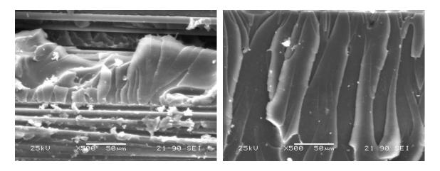
**Fig. 2.** SEM micrographs of the fracture surfaces of the static ENF specimens (CF/EP – left, CF/MWCNT/EP – right)
