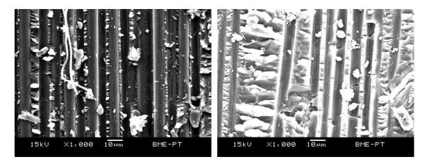
**Fig. 9.** SEM micrographs of the fracture surfaces of the DNS fatigue specimens (CF/EP – left, CF/MWCNT/EP – right)
