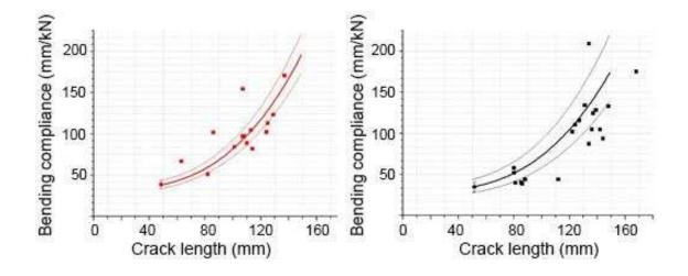
**Fig. 7.** Remaining bending compliance of the failed ENF fatigue specimens (CF/EP – left, CF/MWCNT/EP – right)
