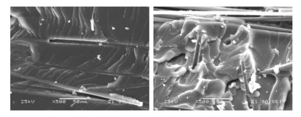
**Fig. 6.** SEM micrographs of the fracture surfaces of the ENF fatigue specimens (CF/EP – left, CF/MWCNT/EP – right)
