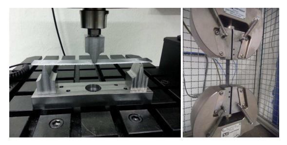
**Fig. 1.** Test setup of the ENF (left) and DNS tests (right)
