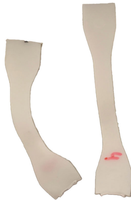
Fig. 5 Heat conditioned 1 mm thick, 1BA samples to check the orientation ( 5 \text{ cm}^3/\text{s} (left), 40 \text{ cm}^3/\text{s} (right))
