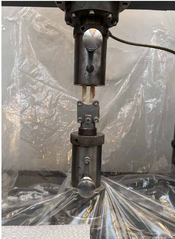
Fig. 1. Measurement arrangement: doubled tendon clamped, frozen with dry ice, and connected to the material measuring device.
