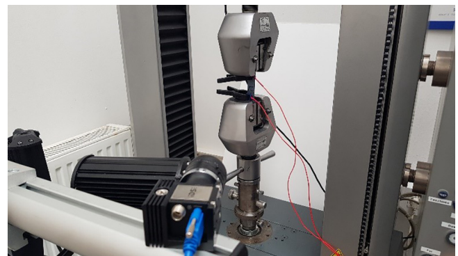
Fig. 2. Test setup of the compression tests.
