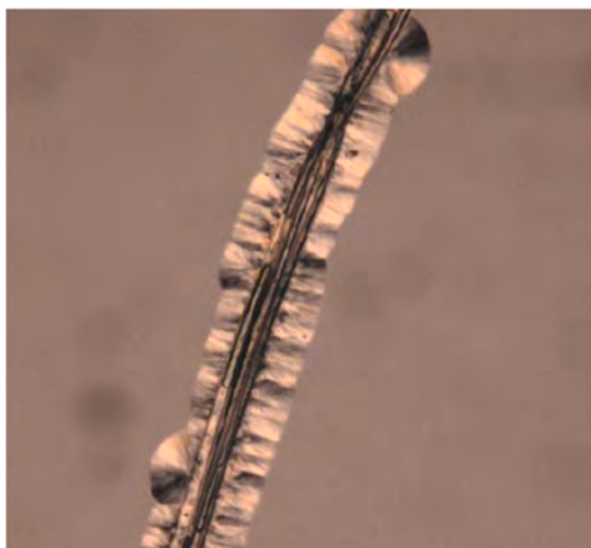
Fig. 38. Optical micrograph of transcrystalline structure around a natural fiber (reprinted from “Y. Wang, B. Tong, S. Hou, M. Li, C. Shen, Transcrystallization behavior at the Poly(lactic acid)/sisal fibre biocomposite interface, Compos. Part A Appl. Sci. Manuf. , 42 (2011), 66–74”, Copyright (2011), with the permission from Elsevier).
