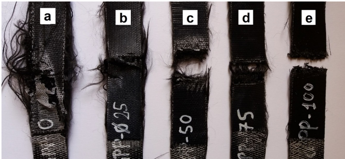
Figure 7. Typical failure behavior of (a) rPP, (b) APAO-25, (c) APAO-50, (d) APAO-75 and (e) APAO.
