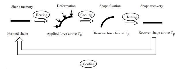
Figure 3. Schematic working principle of shape memory polymers [52].
