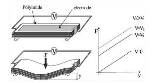
Figure 1. Electro-bonded laminate working principle [31].
