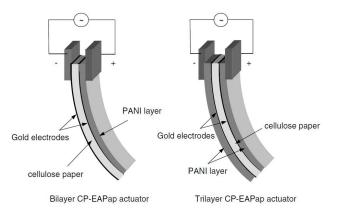
Figure 2. Bi- and trilayer polyaniline coated electroactive paper actuators [32].
