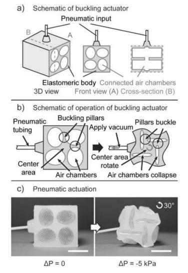
**Figure 5.** Schematics of a pneumatic buckling actuator. (**a**) actuator structure, (**b**) actuator operation, (**c**) pneumatic actuation [73].
