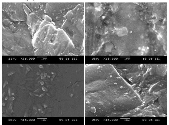
Fig. 5 Cryofractured surfaces of matrix (top left), 10 wt% CBT 100 blend (top right), 20 wt% CBT 100 (bottom left) and 10 wt% CBT 160 (bottom right)
