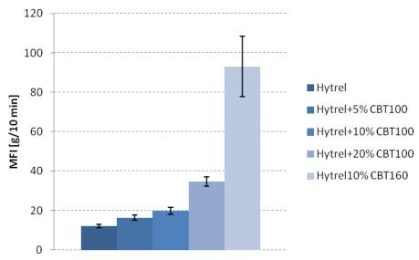
Fig. 2 Melt flow index of the different blends (at 190°C with 2.16 kg load)
