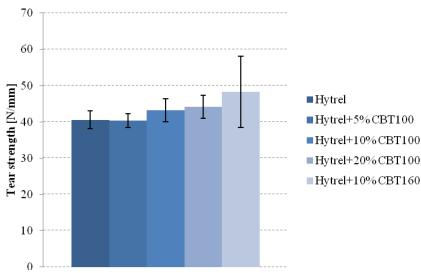
Fig. 4 Tear strength of the different blends
