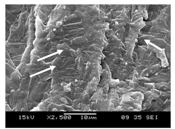
Fig. 6 Disc-like CBT domains in the TPE with 10 wt% CBT160 (arrows indicate)
