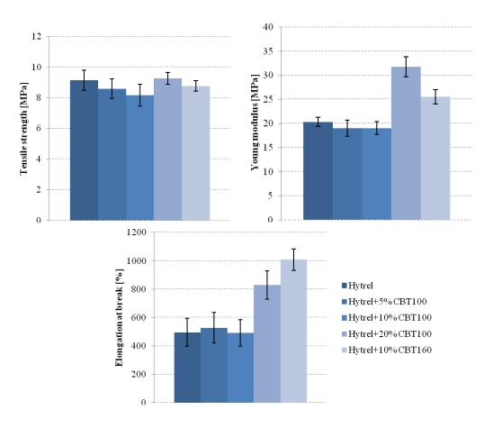
Fig. 3 Static tensile properties of the different blends
