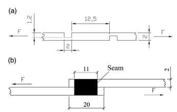
**Figure 3.** Side view of the test specimens used in the shear strength tests. (a) Test specimen made of APPC raw material, prepared according to ASTM D3846 and (b) welded sample prepared for the lap shear strength test.
