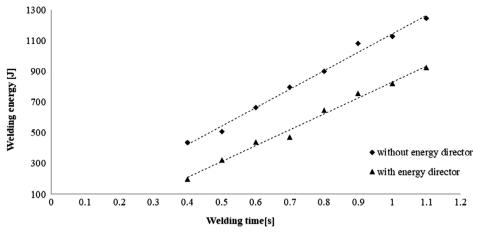
Figure 7. The energy necessary for welding with and without an energy director, as a function of welding time.
