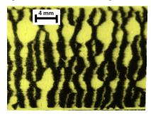
Figure 7. Microscopic images from the surface of a typical tested sample, interrupted before final failure, showing the fragmentation path and delaminated areas around the cracks.
