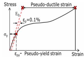
Figure 2. Schematic of the typical stress–strain graph of a thin-ply hybrid with pseudo-ductility.
