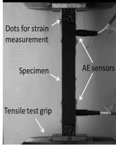
Figure 4. Schematic of the experimental setup, schematic and experimental picture.
