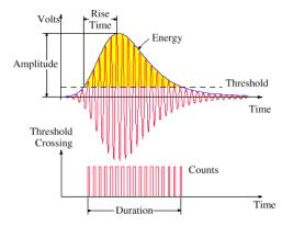
Figure 5. The definitions for acoustic-emission parameters [36].
