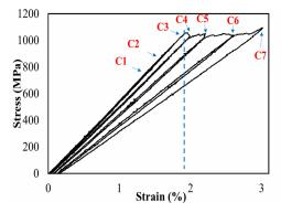
Figure 8. Stress-strain curve for a typical specimen subjected to cyclic loading. The dashed line corresponds to the damage initiation.
