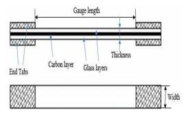
Figure 3. Specimen schematics.
