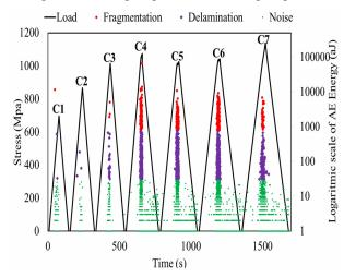
Figure 9. Stress-time and distribution of AE event energy for the hybrid laminate.
